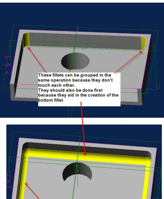
Bottom fillet was created in one pass Another example of using fillets properly is shown in the examples below.
